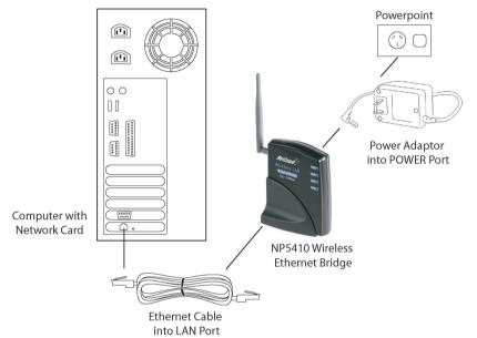
1. Connect your NP5410 to a computer or switch directly using the supplied Cat-5 ethernet cable.
